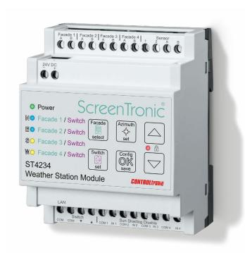
Weather Station Module ST4234 for recording and forwarding of weather information (GPS, sun position, brightness, rain, wind, temperature) from the weather station sensor ST4281 to the local network (LAN) for the subsequent display and processing in the Blind Control Center ST41xx.
